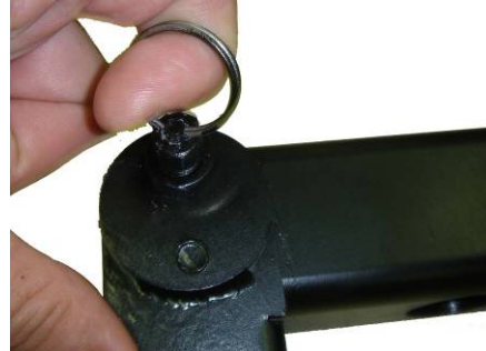
(2) Release pivoting arm locking pin
