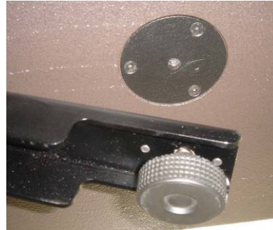
(6) Rotate the pivoting arm into position
