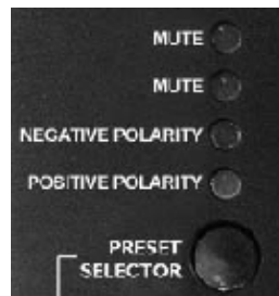
Figure 8: SB15P preset selector switch closeup
